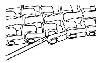
2. Release the screwdriver to expose the rod end.
