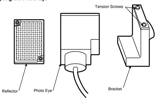
If the beam is not properly lined up on the reflector, the output and signal lights will not be illuminated. To adjust the beam into the reflector, loosen the two tension (Phillips) screws on the top of the mounting bracket (see the illustration above) and move the eye by hand until the red light is centered on the reflector.
