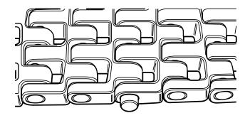
3. Use a pliers, pincer, or similar tool to pull the rod out completely. When grasping and pulling the rod, be careful to not cut or break off the exposed outer finger.
