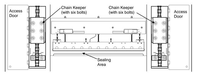
4. Temporarily remove the chain keepers: use a ¼ inch hex wrench to loosen the bolts securing the chain keepers. There are six (6) bolts on each side of each of the chain keepers.
