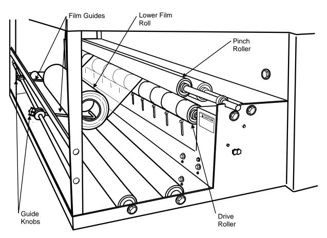
3. Place the film on the support rollers with the film coming off the bottom as shown.
