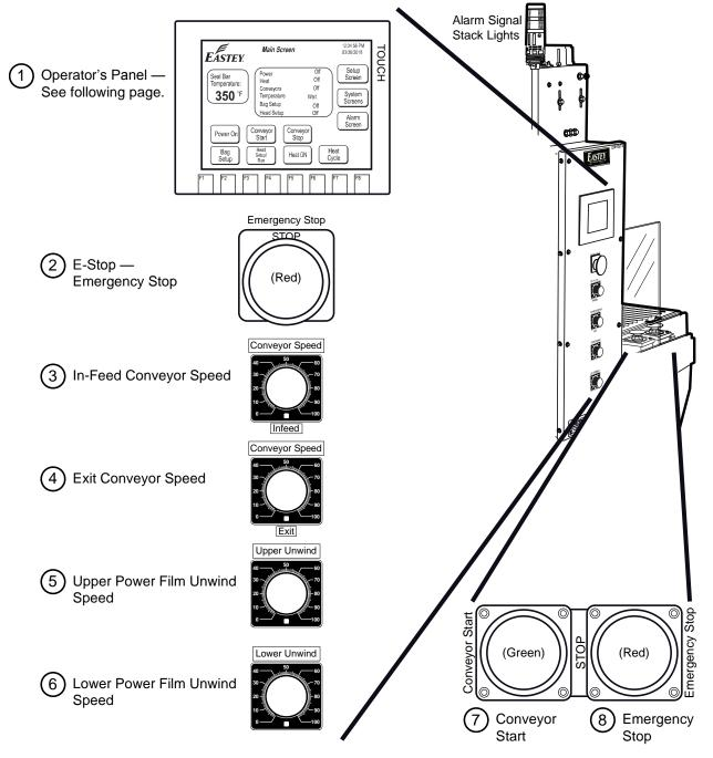
Controls for the automatic bundler are located along the side of the machine as shown in the above figure. Controls listed top to bottom above are explained on the following page. 1. **Operator's Panel** — The operator's panel is a fully-functional color touch screen. It displays current status information and displays buttons for configuring and controlling the system. The Main Screen of the panel interface is shown here.
