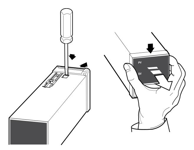
For the second option (to replace entire controller and receptacle), first take note of wire locations (make a sketch and label the wires with tape, if necessary), and then disconnect wires from the temperature controller and thermocouple. Slide the controller and receptacle out of the front of the panel. Replace with a new controller and reconnect wires to the temperature controller and thermocouple. (Refer to notes made during disassembly or the electrical schematic if necessary.)
