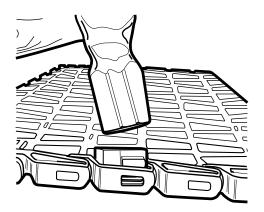
3. Use a flat-blade screwdriver to give the retainer clip a "double click" to finish seating it in place
