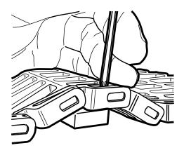
2. Use a screwdriver to push down on the retainer clip to unseat it.
