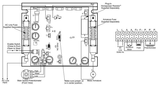
CONTROL LAYOUT & GENERAL CONNECTION DIAGRAM (Model KBMM-225D Shown) (Note: Control is set for 208/230 VAC line input, 0-180 VDC output with armature feedback)
