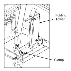
Remove the case and loosen the clamp that is located at the base of and in front of the minor (short) flap folding tower.
