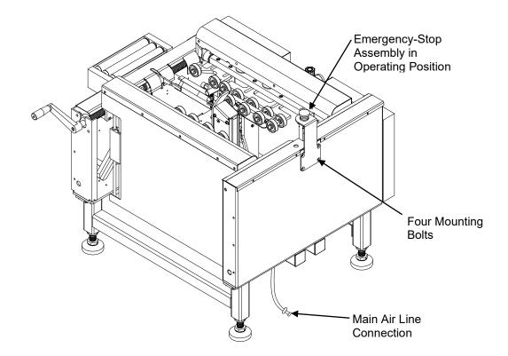
After the E-Stop button has been mounted in the operating position, making sure the red emergency e-stop button is pressed down (off), connect the two air-lines to the E-Stop assembly.
