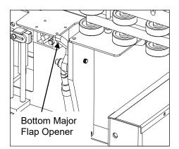
2. The two small levers of the major (side) flap openers momentarily open the bottom major flaps wider to clear the minor (end) flaps.
