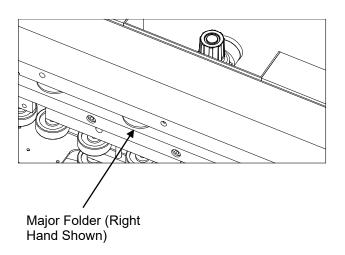
4. The major flap folders then fold up both side flaps of the bottom and stay in position to support the box for packing.
