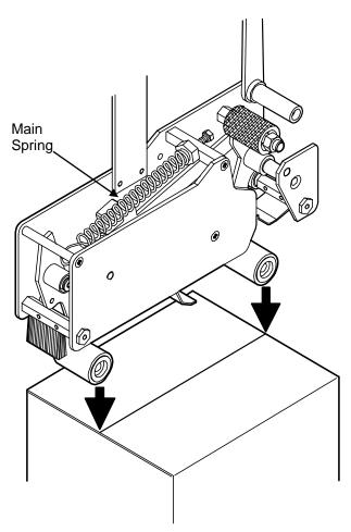
For sealing light weight boxes, decrease the main spring tension. For heavier boxes, increase the main spring tension.
