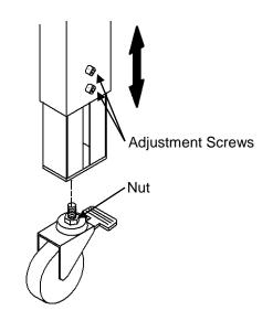
CAUTION! The case taper must be lifted off the floor to install the casters. Use proper equipment when lifting the case taper. Ensure the SB-Ex Ran Case Taper is secure and will not shift while installing the casters or adjusting leg height.
