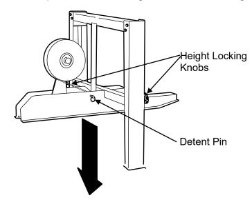
Lift the upper cartridge up and out of the machine.
