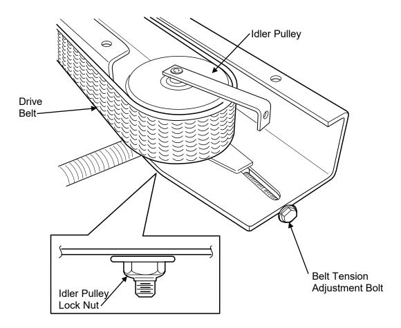
Loosen the idler pulley locking nut located under the idler pulley
