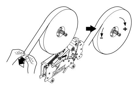
Check the tape for correct tension. If the tape head used with the taper allows for adjustment of tape tension, tighten or loosen the tape core holder to adjust to correct tension.
