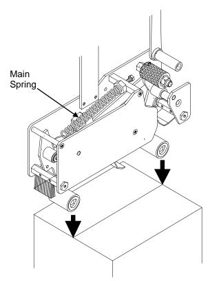
For sealing light weight boxes, decrease the main spring tension. For heavier boxes, increase the main spring tension.
