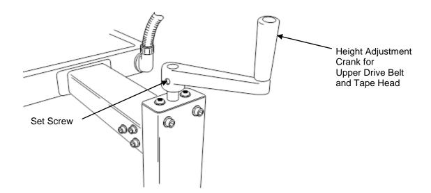
The height adjustment crank can be mounted on either side of the machine by loosening the set screw, removing the crank, and mount to the crank onto the adjustment spindle on the opposite side of the machine. Re-tighten the set screw to secure the adjustment crank.
