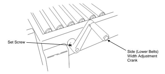
The side belt width adjustment crank can be mounted on either side of the machine by loosening the set screw, removing the crank, and mounting the crank on the opposite side of the machine. Re-tighten the set screw to secure the adjustment crank.
