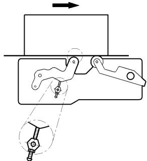
Check tape tension set by the spring tension at the tape core.
