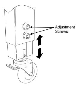
**CAUTION!** Ensure the case taper is secure and will not shift while adjusting leg height.
