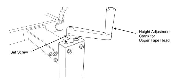
The height adjustment crank can be mounted on either side of the machine by loosening the set screw, removing the crank, and mounting the crank onto the adjustment spindle on the opposite side of the machine. Re -tighten the set screw to secure the adjustment crank.
