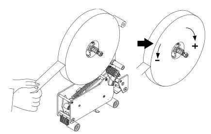
Check the tape for correct tension. Tighten or loosen the tape core holder to adjust tension.
